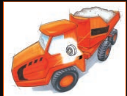
Turning ring placement in front of the articulation point provides equal weight distribution to each front wheel at all times.
